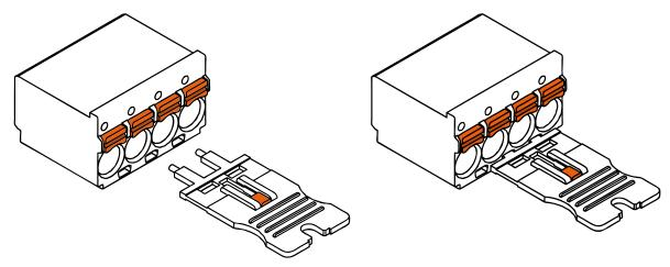
\*NB – Use of the strain relief clip is optional, however it is required in order to remove the screwless header from the screwless connector.
