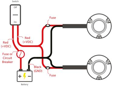
The light cables can be extended. Ensure the correct cable gauge is used to avoid issues with voltage drop. Follow ABYC recommendations for no more than 3% voltage drop for 12 VDC, and 10% for 24 VDC installations. Consult a qualified electrical installer, or contact Lumishore for further information.
