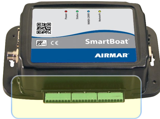
Figure 3-1: Pluggable terminal blocks for device connections
