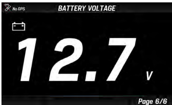
Layout SINGLE : single box. The data value is numeric or displayed by a gauge.
