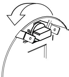
Remove lamp & replace with # 40102E007 and #6283274 socket.
