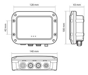
Figure 4 AIS antenna splitter dimensions
