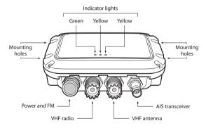
Figure 2 AIS antenna splitter overview
