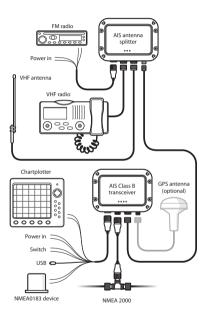
Figure 3 Typical installation configuration
