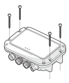
Figure 5 AIS antenna splitter mounting
