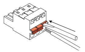
Release the orange button to lower the clamp on to the wire strands for a secure termination.
