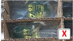
Smaller sections with a SINGLE unit per section offers the *better* protection. Larger sections with two or more units per section are much more prone to material movement and subsequent damage during delivery.
