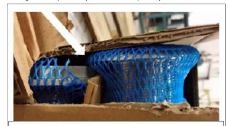
Besides the container damage, the internal divider used here was not able to prevent metal housings from contacting and then damaging each other. The blue fishnet material did not prevent damage.
