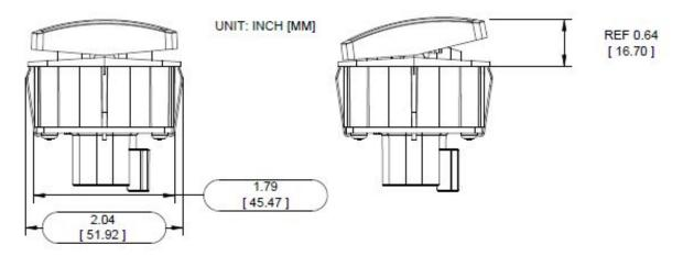
Figure 3 - Hardware Description Side View
