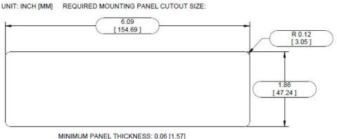
Figure 6 – Mounting Panel Cutout Dimension
