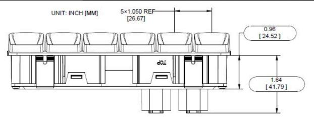
Figure 2 - Hardware Description Top View
