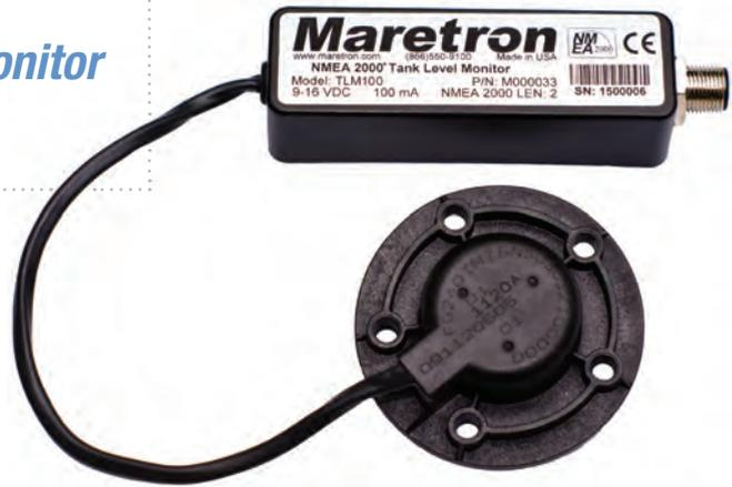
The TLM100 is mounted directly to the top of tanks using the industry standard SAE J1810 5-hole mounting pattern. The TLM100 can also be mounted to tanks with threaded tank openings using optional adapters that included both a 1.5" NPT and a 1.25" BSP adapter. There are other important TLM100 optional accessories including an optional focus tube to permit use on boats with planing hulls, which is required if the vessel spends a significant amount of time with the bow pitched up.
