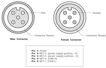
Figure 2 – NMEA 2000<sup>®</sup> Connector Face Views
