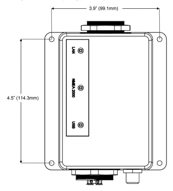
Figure 4 - Mounting Surface Template
