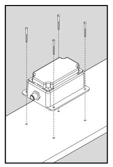
Figure 1 – Mounting the DCM100
