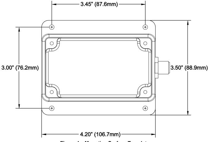
Figure 4 – Mounting Surface Template
