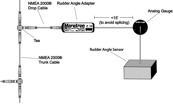
Figure 1 – Mounting Location When Used with Analog Gauge
