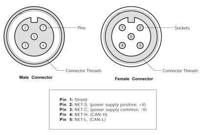
Figure 4 – NMEA 2000<sup>®</sup> Connector Face Views
