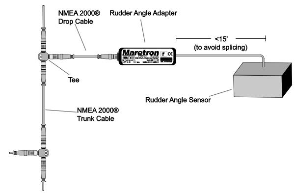
Figure 2 – Mounting Location When Used Without Analog Gauge
