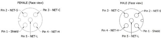
An Actisense Panel Mounted Wire (PMW) connector is a great tool for plugging in to a spare T-piece to quickly identify the correct pins via the wiring colours. It is recommended that each wire from the PMW is terminated inside a terminal block prior to plugging it in to the network as voltage may be present across the NET-S and NET-C pins
