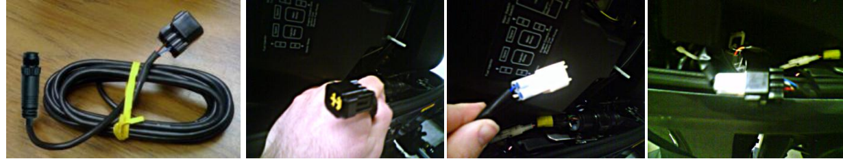
1) Interface Cable, p/n: 000-0120-37 2) Adapter installed in cowling. 3) Yamaha 4-pin connector. 4) Completed connection.
