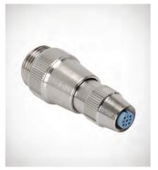
The reducer is used to change from a Mini cable to Micro or Mid cable. For example, one end of the network might be terminated at the top of the mast but it may not be desireable to run a Mini trunk cable up the mast. In this case, you can switch over to Micro or Mid cable at the base of the mast using the reducer and continue up the mast with Micro or Mid cable.
