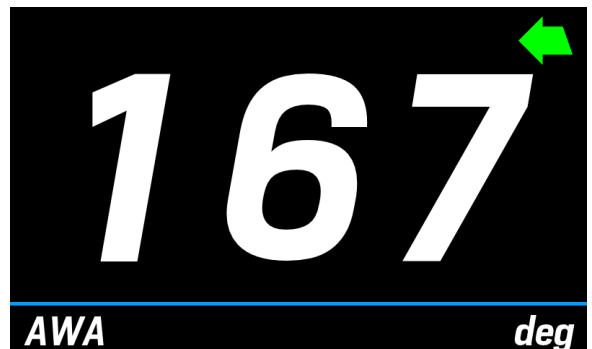
Layout MAST : four pages with data about: Apparent wind angle (AWA) , Apparent wind speed (AWS) , Speed through water (STW) , True heading .
