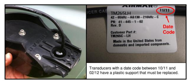
**Upgrade Stock and In-field Repair:** All affected stock must be updated. Please contact Airmar to make arrangements for a replacement plastic transducer support.
