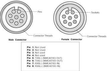
Connect the other end of the cable consisting of individual wires using recommended practices for installing NMEA 0183 products. Please note that NMEA 0183 does not have a standard for connectors and the customer/installer should contact the manufacturer of the equipment to which the compass is being connected for information on how to properly connect the device to the compass. The individual wires found within the cable have the following color coding:
