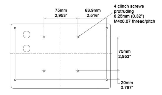
Figure 3 – TSM810C VESA Arm Mounting Retention Screws
