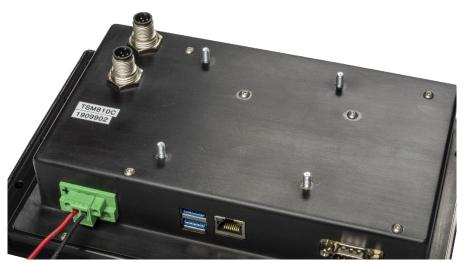
Figure 4 – TSM810C VESA Arm Mounting Retention Screws
