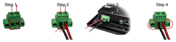
Figure 9 – Attaching Power Cables to Connector
