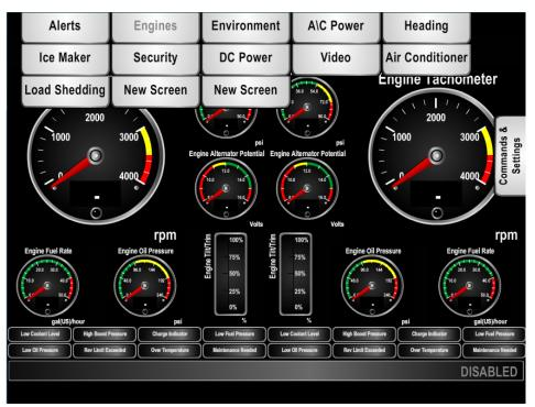
Figure 12 – N2KView<sup>®</sup> Window with Tabs Displayed
