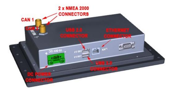
Figure 5 – TSM810C Bottom and Rear Panels
