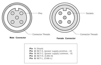
Figure 10 – NMEA 2000<sup>®</sup> Connector Face Views
