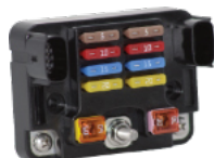
5015 10 Pos Fuse Block 8 ATO + 2 LP-JCase
