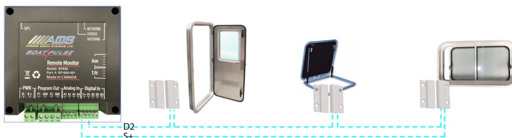
Figure 12 Connecting multiple door magnetic read contact sensor in series (must be NC type)
