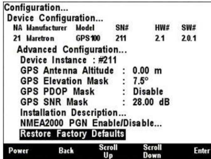
Figure 115 – Restoring Factory Defaults on the GPS100
