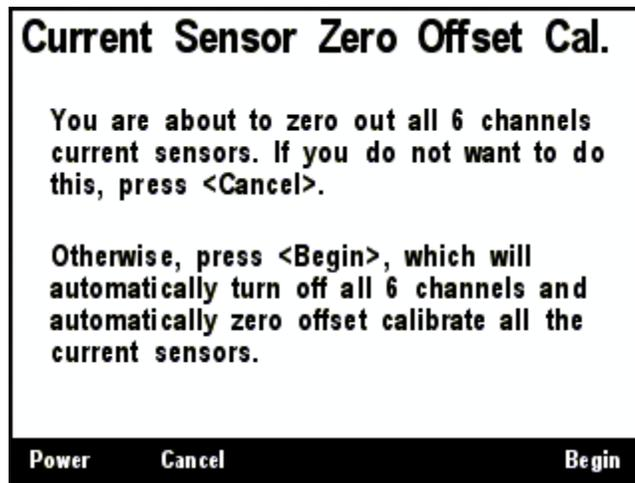
**Figure 53 – DCR100 Current Sensor Zero Offset Calibration Screen**
