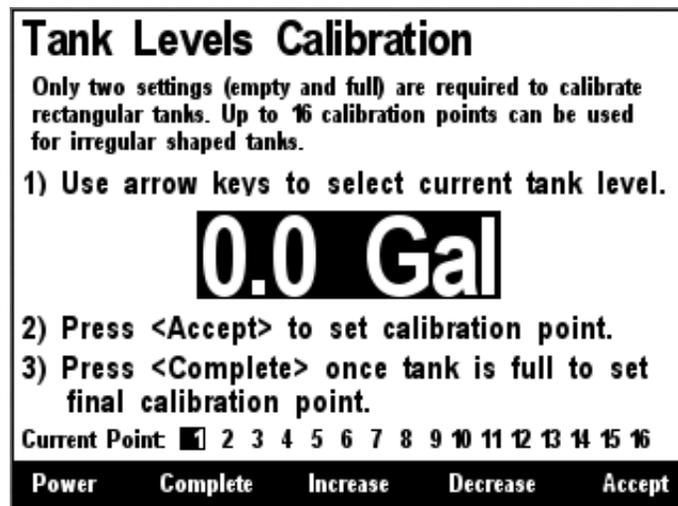
**Figure 209 – Empty Level Calibration**
