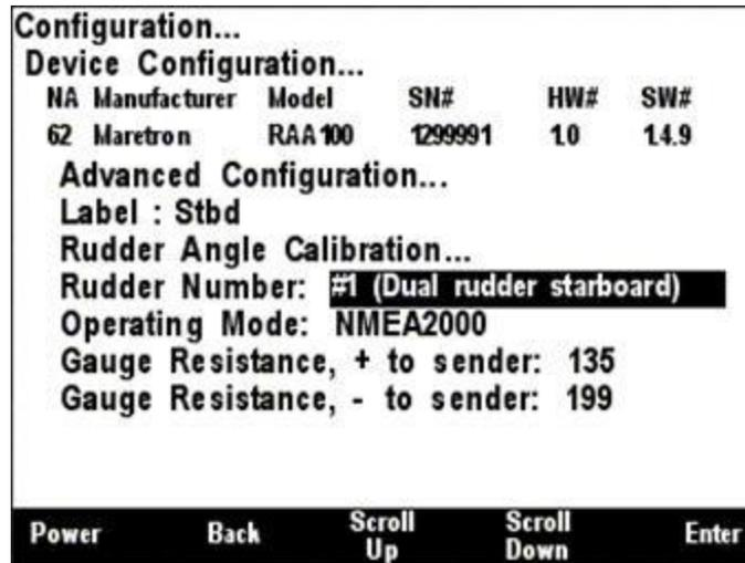
Figure 151 – RAA100: Setting the Rudder Number
