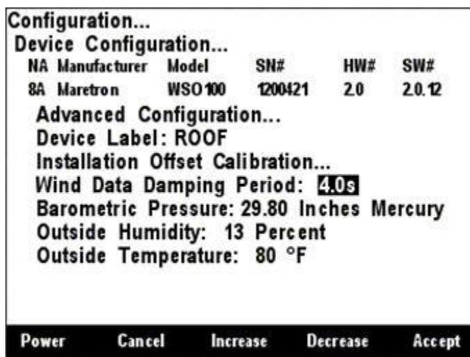
Figure 232 – Setting the Wind Data Damping Period
