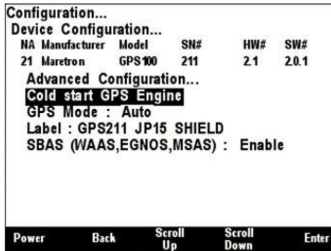
Figure 116 – Performing a Cold Start of the GPS100
