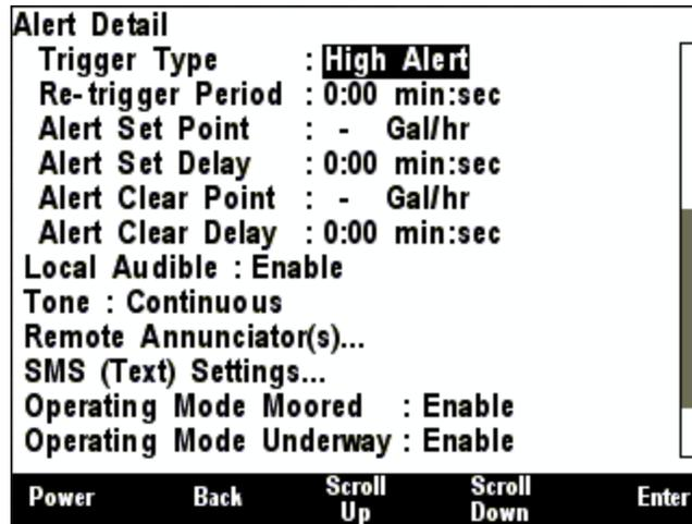
**Figure 277 – Trigger Configuration – High Alert**
