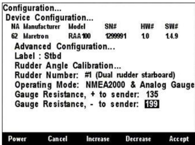
**Figure 154 – RAA100: Setting the – to Sender Gauge Resistance**
