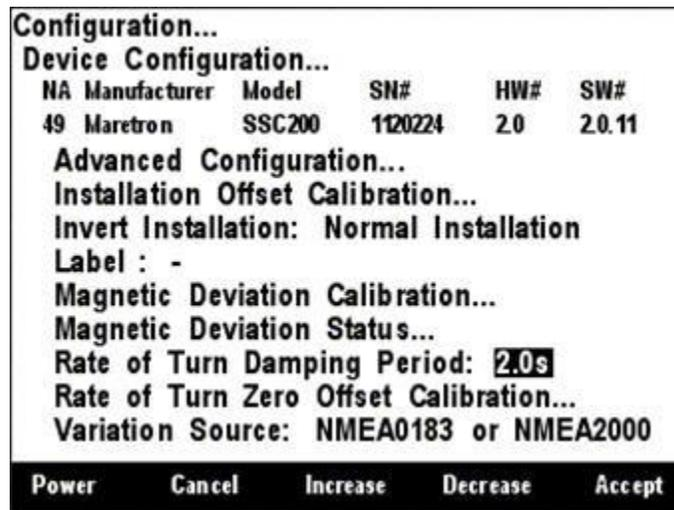
**Figure 178 – Programming SSC200/SSC300 Rate of Turn Damping Period**
