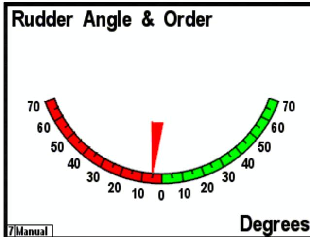
Figure 243 – Rudder Angle Gauge Display Example
