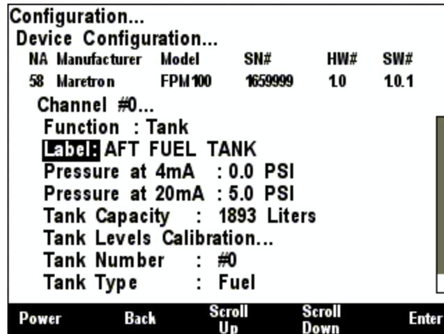
**Figure 98 – FPM100 Channel #0 First Configuration Screen (Tank Mode)**
