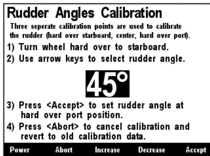
*Figure 147 – RAA100 Starboard Rudder Angle Calibration*
