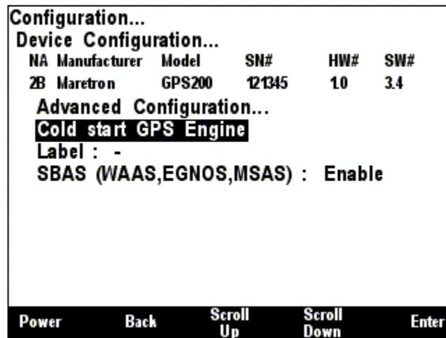
Figure 123 – Performing a Cold Start of the GPS200
