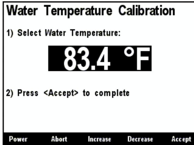
Figure 80 - DST110 Water Temperature Calibration Screen
