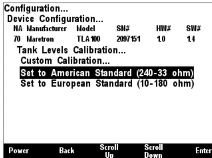
**Figure 195 – American Standard Sender Calibration**
