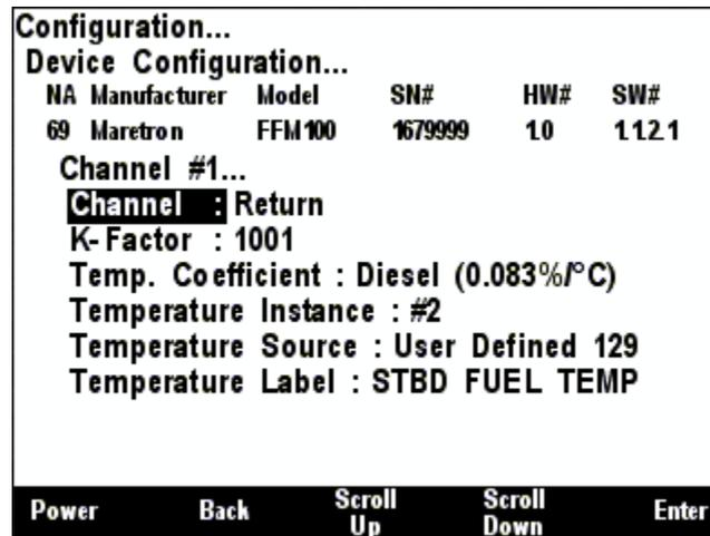
**Figure 92 – FFM100 Channel #1 Configuration Screen (Differential Mode)**
