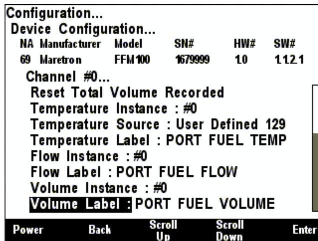
Figure 89 – FFM100 Channel #0 Second Configuration Screen (Differential Mode)
