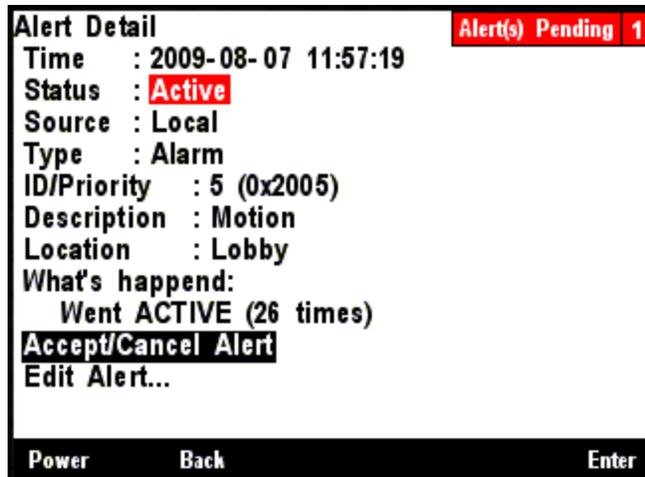
*Figure 273 – The Alert Detail Screen*
