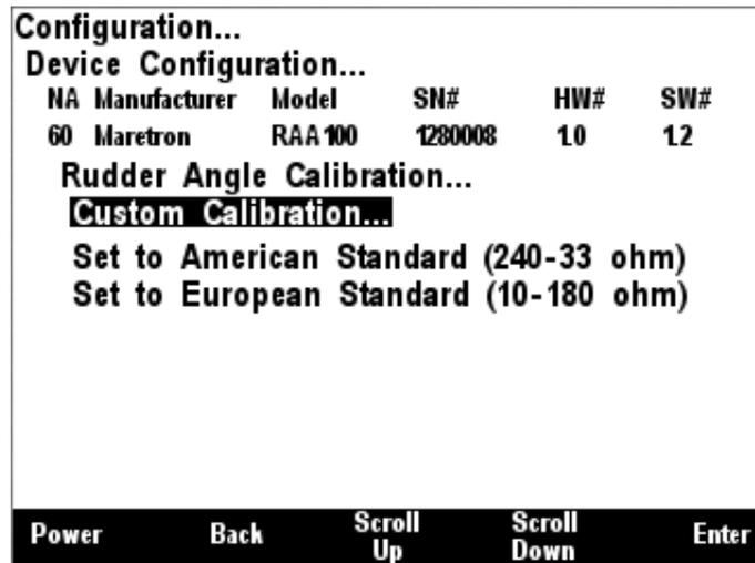
*Figure 146 – RAA100 Custom Rudder Angle Calibration*
