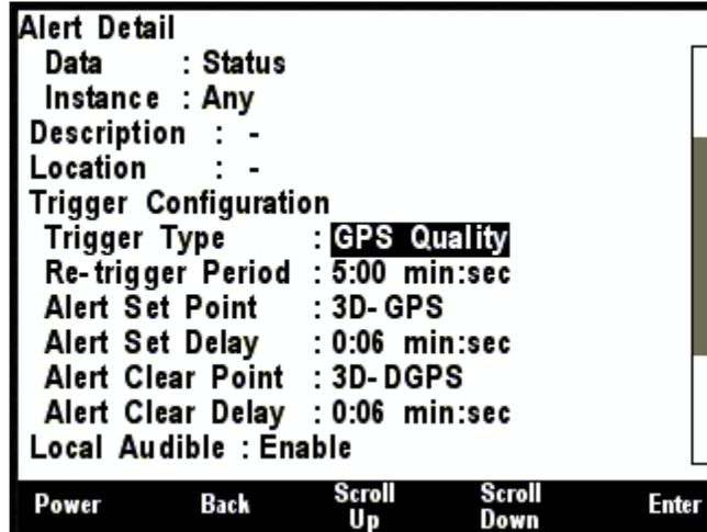
Figure 287 – Trigger Configuration – GPS Quality Alert
