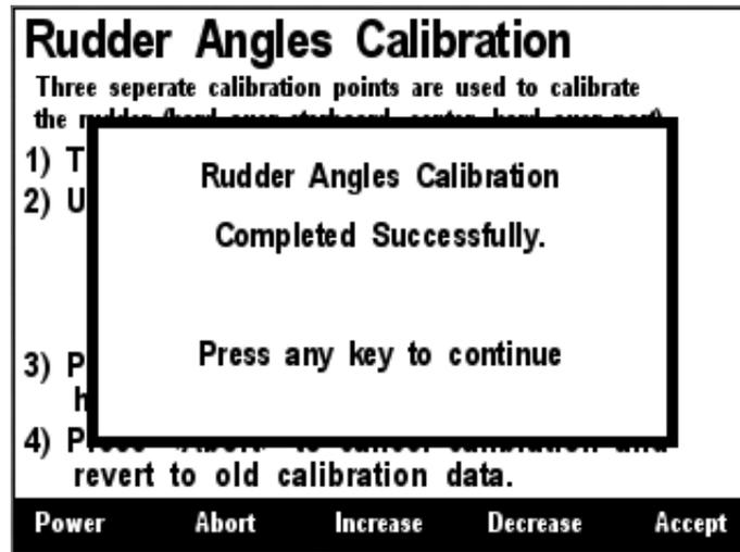
*Figure 150 – RAA100 Custom Rudder Calibration Confirmation Screen*
