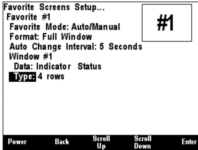
**Figure 246 – Configuration of Indicator Light Display**
