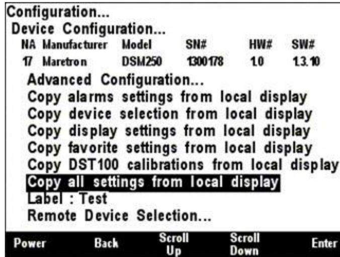
*Figure 68 – DSM150/DSM250/DSM410/DSM570 Copy all settings from local display*
