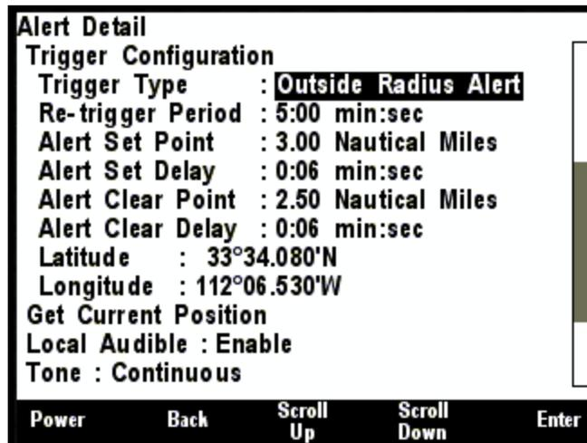
**Figure 285 – Trigger Configuration – Outside Radius Alert**
