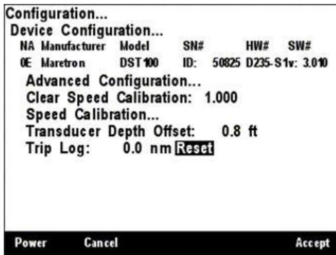
*Figure 75 – Resetting the DST100 Trip Distance Log*
