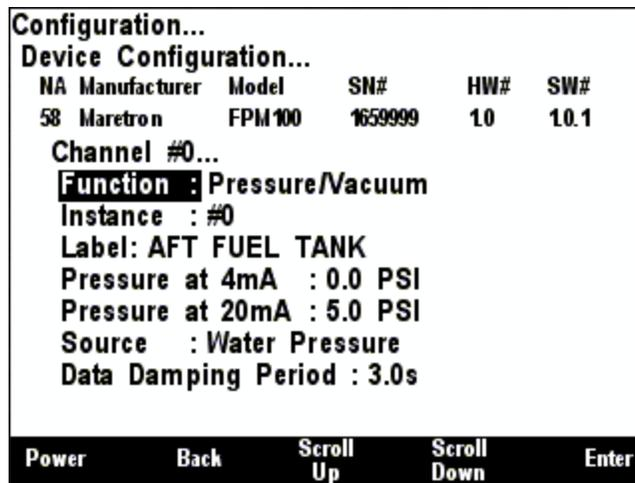
**Figure 107 – FPM100 Channel (Pressure/Vacuum Mode) Configuration**
