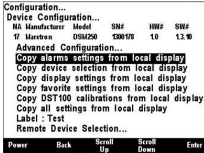
**Figure 62 – DSM150/DSM250/DSM410/DSM570 Copy alarms settings from local display**
