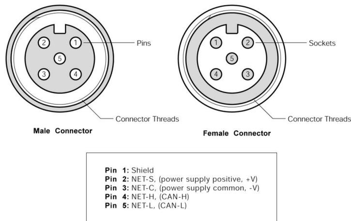
**Figure 1 – NMEA 2000® Connector Face View**
