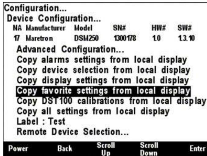
Figure 65 – DSM150/DSM250/DSM410/DSM570 Copy favorite settings from local display
