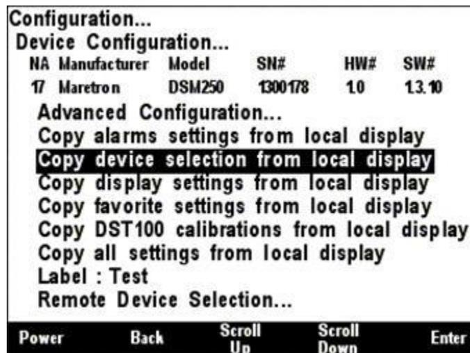
**Figure 63 – DSM150/DSM250/DSM410/DSM570 Copy device selection from local display**
