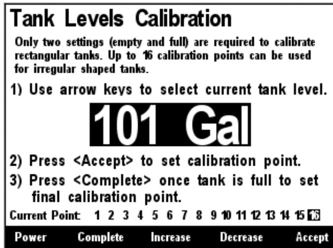
*Figure 211 – Full Level Calibration*
