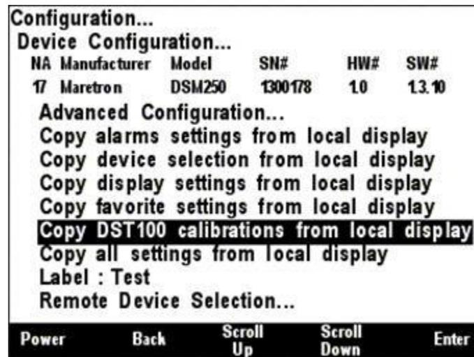
**Figure 67 – DSM150/DSM250/DSM410/DSM570 Copy DST100 calibrations from local display**
