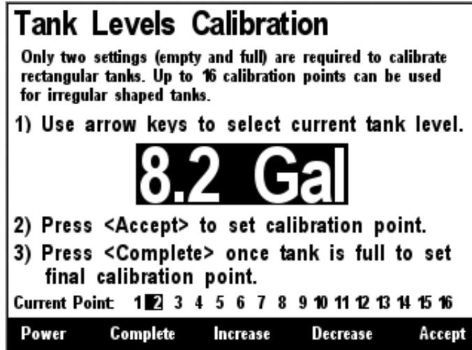
*Figure 210 – Intermediate Level Calibration*
