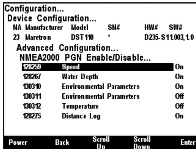
**Figure 78 – DST110 NMEA 2000® PGN Enable/Disable Screen**
