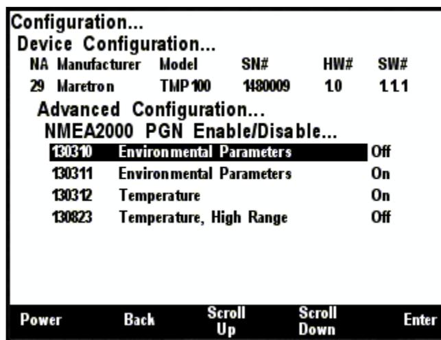
**Figure 217 – TMP100 NMEA 2000® PGN Enable/Disable Screen**
