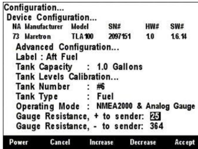
Figure 200 – Configuring the + to Sender Gauge Resistance
