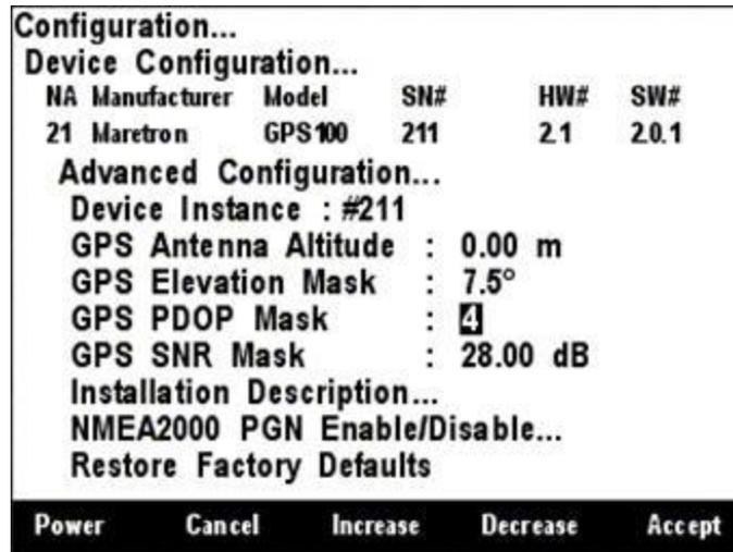
Figure 112 – Configuring PDOP Mask on a GPS100
