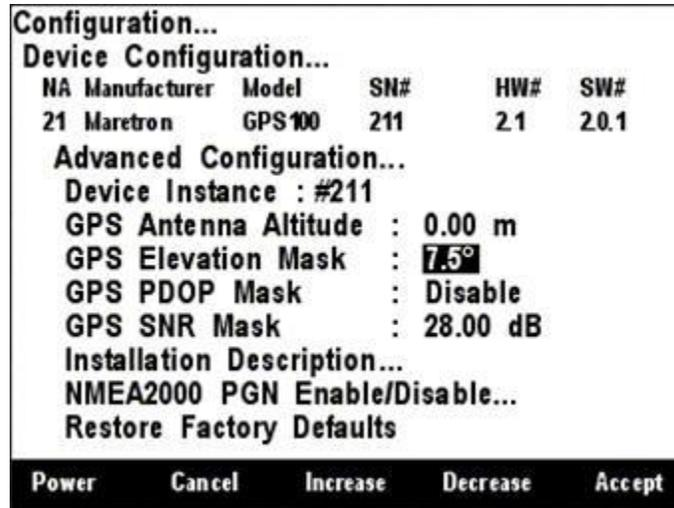
*Figure 111 – Configuring Satellite Elevation Mask on a GPS100*
