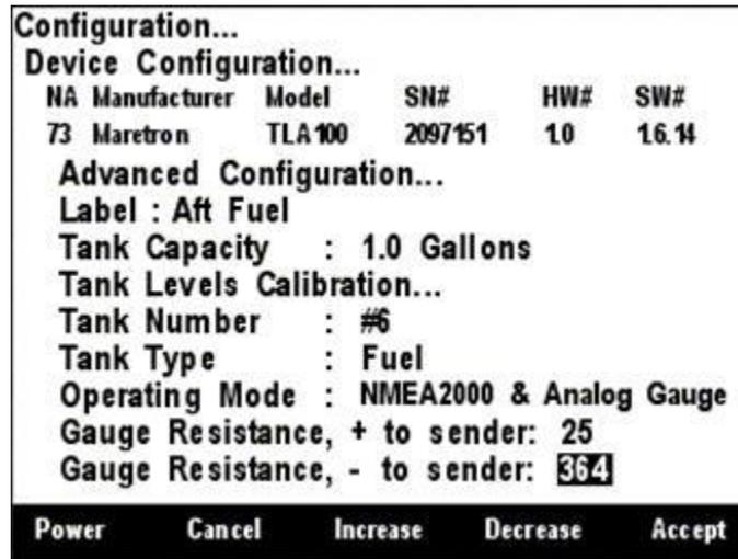
*Figure 201 – Configuring the - to Sender Gauge Resistance*
