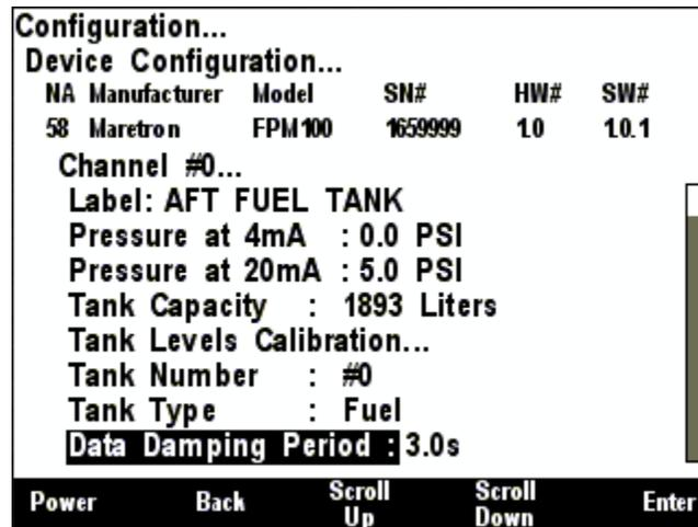
**Figure 99 – FPM100 Channel #0 Second Configuration Screen (Tank Mode)**
