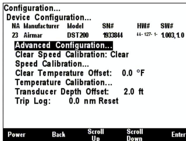
**Figure 30 – Airmar Depth/Speed/Temperature Transducer Configuration Screen**
