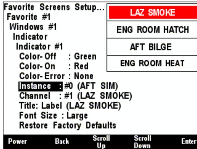
**Figure 248 – Configuration of an Individual Indicator Light**
