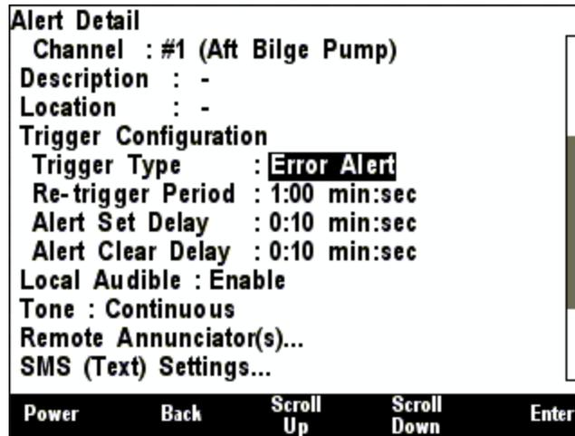
**Figure 283 – Trigger Configuration Editor – Tripped Alert**
