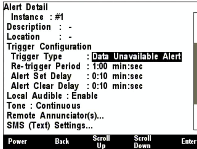
**Figure 280 – Trigger Configuration – Data Unavailable Alert**
