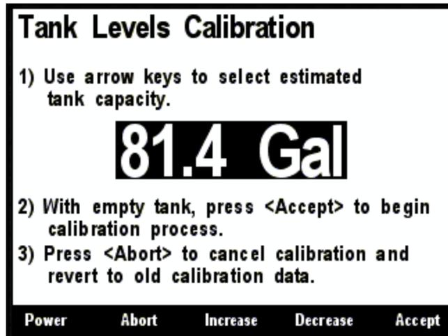
**Figure 208 – Tank Levels Calibration Capacity Estimation**
