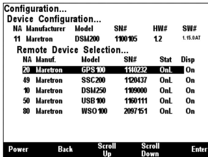
**Figure 59 – DSM200 Remote Device Selection Screen**
