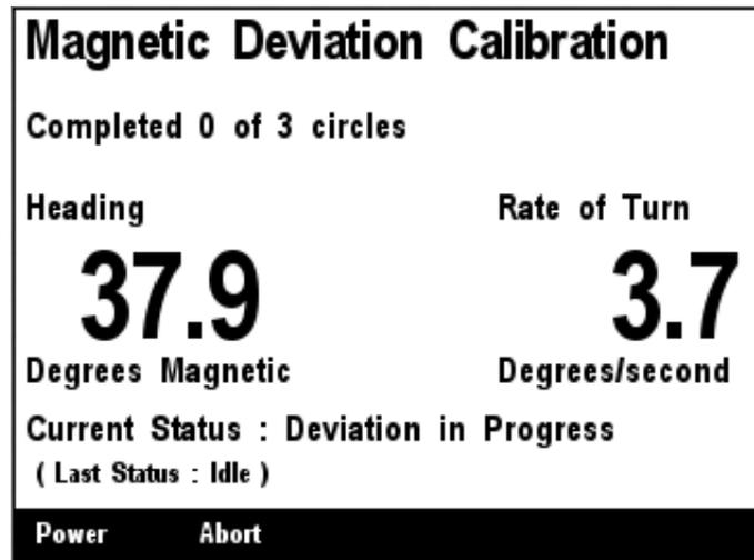
**Figure 176 – SSC200/SSC300 Magnetic Deviation Calibration Progress Screen**
