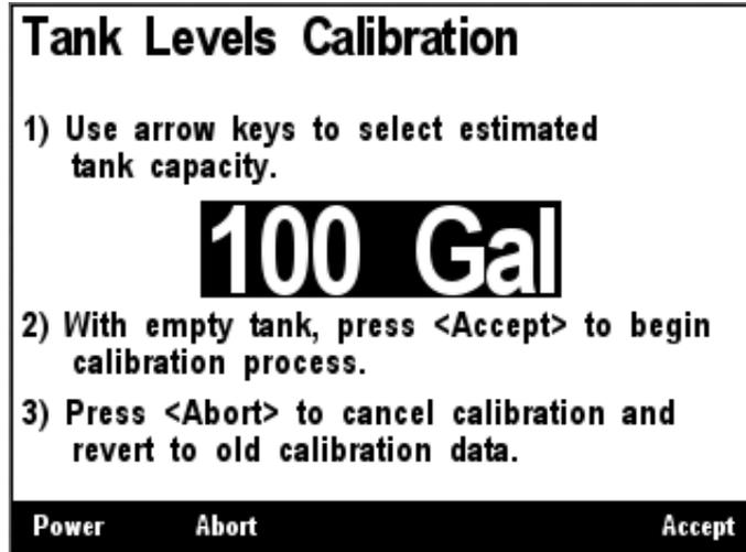
*Figure 101 – Tank Levels Calibration Capacity Estimation*
