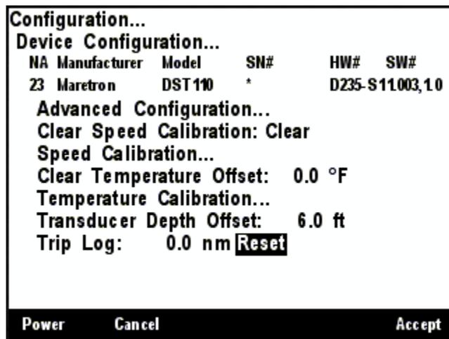
*Figure 82 – Resetting the DST110 Trip Distance Log*
