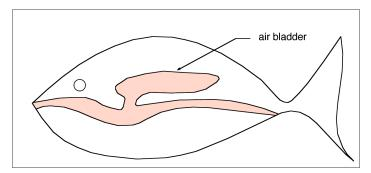
Because the air bladder contains gas, it is a drastically different density than the flesh and bone of the fish as well as the water that surrounds it. This difference in density causes the sound waves from the echosounder to bounce off the fish distinctively. The transducer receives the echoes and the echosounder is able to recognize these differences. The echosounder, then, displays it as a fish.
