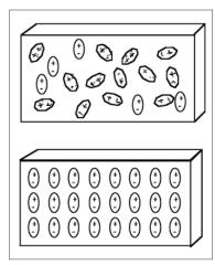
individual crystals that have a positive (+) and negative (-) electric charge on respective ends. These crystals are normally resting in a haphazard way in the piezoceramic element. But if a high voltage electric current is applied to the element, the crystals will adjust their alignment until nearly all are positioned in straight columns with their positive (+) and negative (-) poles lying in the same direction.
