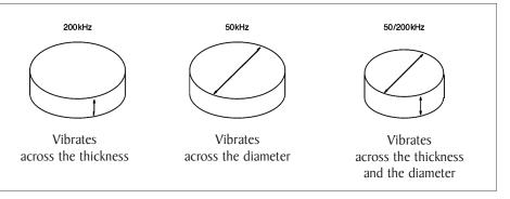
diameter which is called the radial mode. A transducer that can operate at two frequencies will have the characteristics of both frequencies—the ability to "see" well in both shallow and deep water with good bottom definition.
