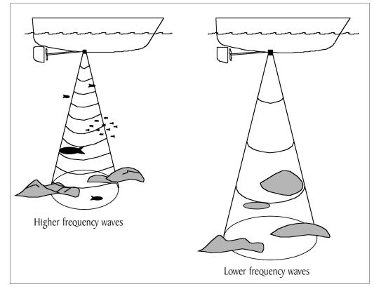
The speed of sound in water is 4,800 feet per second. If we have a 200 kHz transducer then our equation would look like this:
