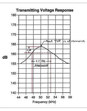
the resonant frequency is divided by the bandwidth giving us a "Q" factor of 9.6. (50 kHz  $\div$  5.2 kHz = 9.6).
