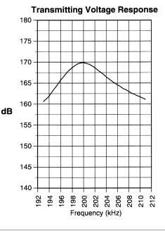
This information is known as performance data which is made available to customers and used as the standard for final testing of the product. The figures are extremely important to our OEMs as this data is used to determine the frequency at which the echosounder must be set.
