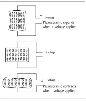
resonant frequencies. The size, shape, and thickness of the piezoceramic element determine the frequency at which it will vibrate best. Engineers very carefully control these factors to produce transducers that resonate at the correct frequency to meet the customers' needs.
