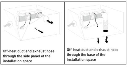
The waste gases (including condensation) can be conducted into the open air or, on yachts, into the bilge.
