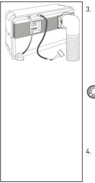
Use a suitable sealant to seal the hole. Ensure that the exhaust hose has no kinks or blockages and that the waste gases can flow freely out of it. Please also pay particular attention to the information about siphoning in the chapter entitled "Important guidelines on choosing a location for installation" on page 10.
