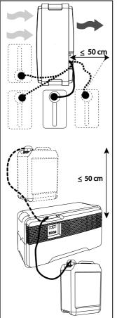
When positioning the fuel cartridge, please ensure that it is within reach of the fuel cartridge connection. The connection hose is 50 cm/20 in long and must not be kinked or pinched at any point.
