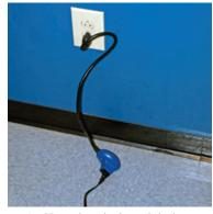
Load Tester plugged in-line with the device
