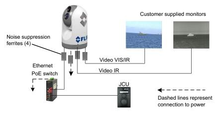
Figure 1-1: Basic installation using a customer PoE switch
