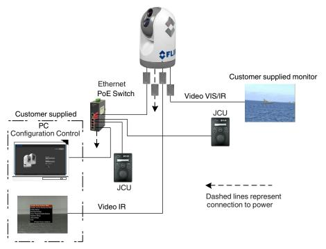
Figure 1-2: Two station installation with a PC
