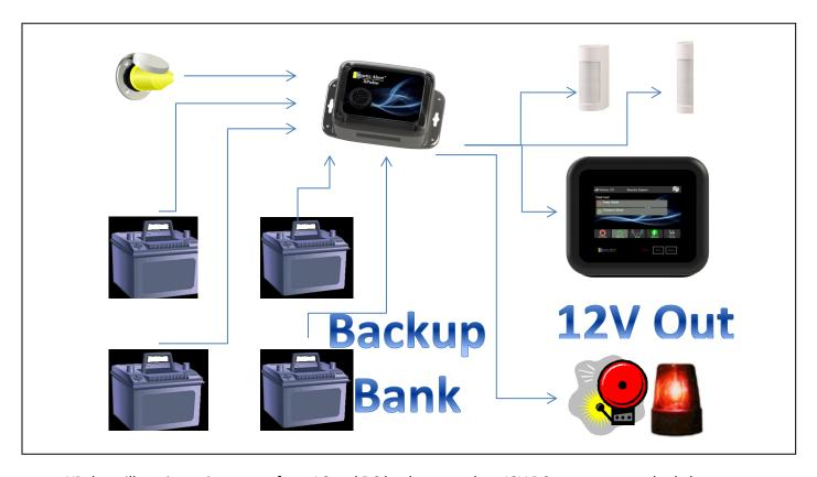
XPulse will use incoming power from AC and DC banks to regulate 12V DC output to attached alarm sensors, optionally for \*powering Insight with battery backup, and for powering the \*integrated siren or an externally attached siren/alarm. In this way, it's possible to add one or more backup batteries dedicated to powering alarm sensors and XPulse for full power fault redundancy and backup, as well as audible and visual alarms throughout the boat.
